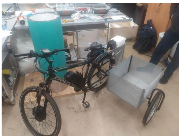
Fig.2 The photo of Riksza H2 - a prototype research platform for zero-emission electric transport with a hydrogen fuel cell stack.
