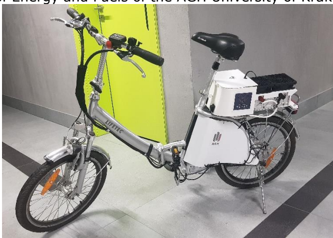
Fig.1 The photo of an electric bicycle powered by a hybrid energy source with PEMFC hydrogen-oxygen fuel cells
